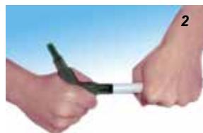
2 Calibrate the pipe to make the position of the fitting easier.
